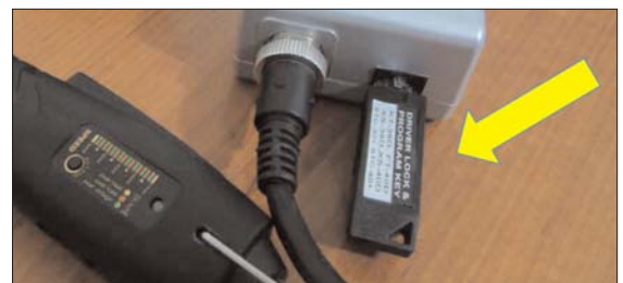
To adjust the settings the Program Lock Key must be plugged into the STC40 Transformer.
